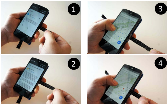
Figure 14: (1–2) Users can switch between the contacts without cluttering the screen, but also (3–4) pan & zoom into maps efficiently by using a bi-manual approach.
