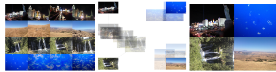
Figure 11: A photo album digest. The input collection of 16 images (left) is reduced to 4 representative images (right). We extend our bipartite matching algorithm to allow n -to- k matching, such that n > k . Middle: the input images, as placed by Isomap (transparent images) and the four selected images in their target grid locations (opaque images). Note our method keeps one image from each group of four similar images.
