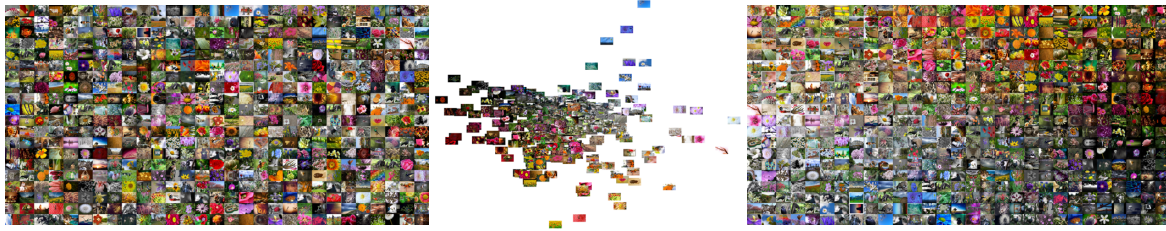
Figure 1: Images of flowers from Flickr. Left: Random ordering makes image set hard to understand. Center: Isomap preserves structure but is poor for page layouts. Right: Arranged by our algorithm using the L2 distance between mean RGB values. Note that good results are obtained even with such a simplistic feature (three values per image).
