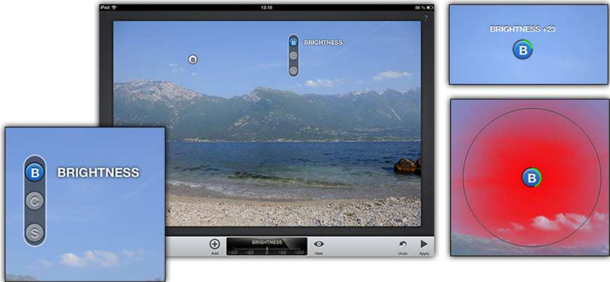
Figure 4. The mobile UI by example of the Selective Adjust module of Snapseed iOS. The main display is shown in the middle. On the bottom of the main display there are controls to add control points, display the value of the currently selected slider, hide all control points, and final application and exit (from left to right). Top right: Transient view of control point during a strength change. Bottom right: Transient view of control point during a size change; the effect strength is visualized by a red overlay. Bottom left: Transient view of a filter change (enlarged section from main image).
