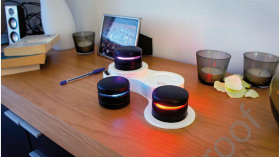
Fig. 4.6 The fully functional final prototype displayed above had three messaging tokens and a simplified docking station
