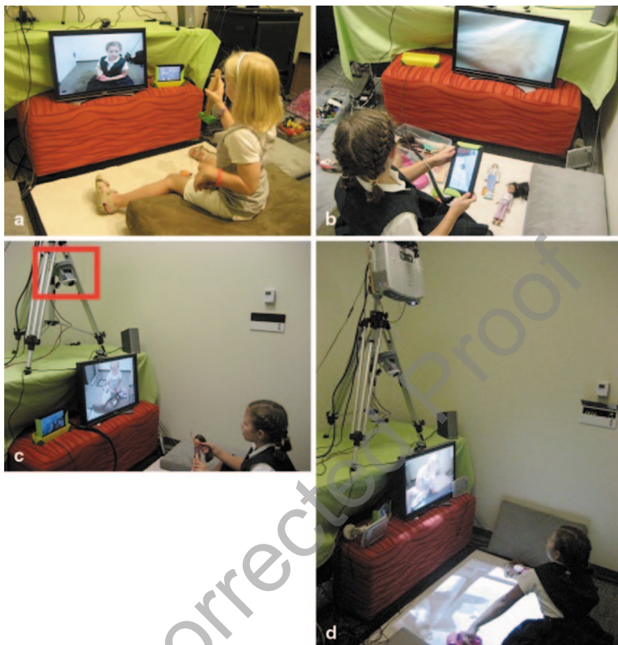
Fig. 6.2 Four video conferencing prototypes tested in Video Playdate research. a Vanilla prototype . The small screen shows what the remote participant sees. b Mobile prototype . Unlocking the small screen activates the camera on the back of the device, allowing the child to control the remote participant's view. c Smart Pan-Zoom-Tilt prototype . A researcher controlled the pan-zoom-tilt camera (red box), allowing the child to request different remote views. d Play Rug prototype . A floor mat is used as the projection surface for a monochrome view of the remote participant's rug
