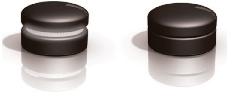
Fig. 4.7 A visualisation of the messaging token. The left token shows the light ring, that is covered in the right one when the token is pressed to play a message
