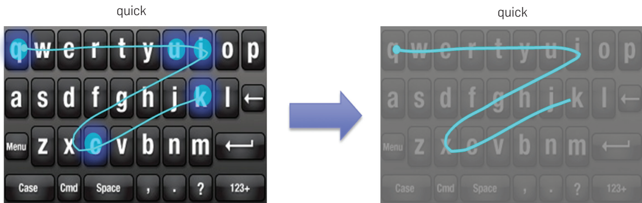
Figure 3. Illustration: word-shorthand gesture keyboarding is expected to shift from primarily visual-guidance driven letter-to-letter tracing to memory-recall driven gesturing.
