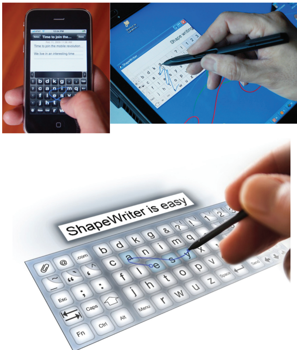
Figure 2. Word-gesture keyboards can also work on alternative keyboard layouts. Shown here are ShapeWriter ATOMIK mode on the iPhone (circa 2008 top left), ShapeWriter on a Windows Tablet with the ATOMIK layout (circa 2005, top right), and an illustration of the ATOMIK layout (bottom).
