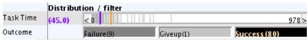
Figure 6: Distribution/Filter Panel. The continuous attribute Task Time is represented by a double-slider bar for filtering with the distribution displayed as a stripe graph on the slider bar. The categorical attribute Outcome is represented by a series of toggle buttons for filtering, with the category name and count as labels, and the counts encoded with luminance in the button background.
